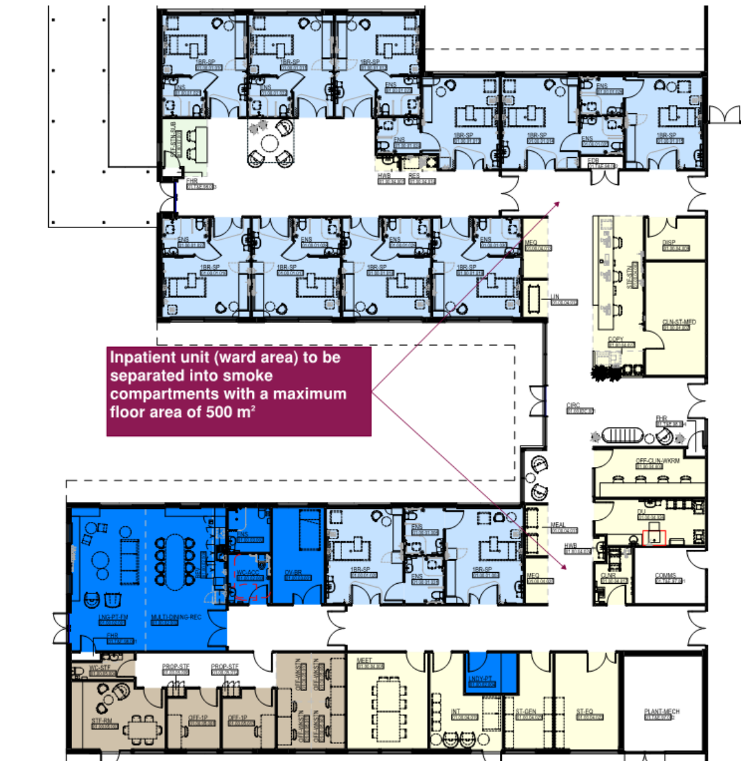
Figure No. 6: Required smoke separation within the proposed inpatient unit.
