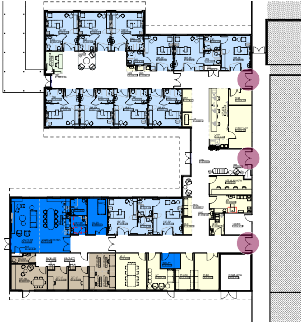
Figure No. 16: Swing of horizontal exit doors against the direction of egress
