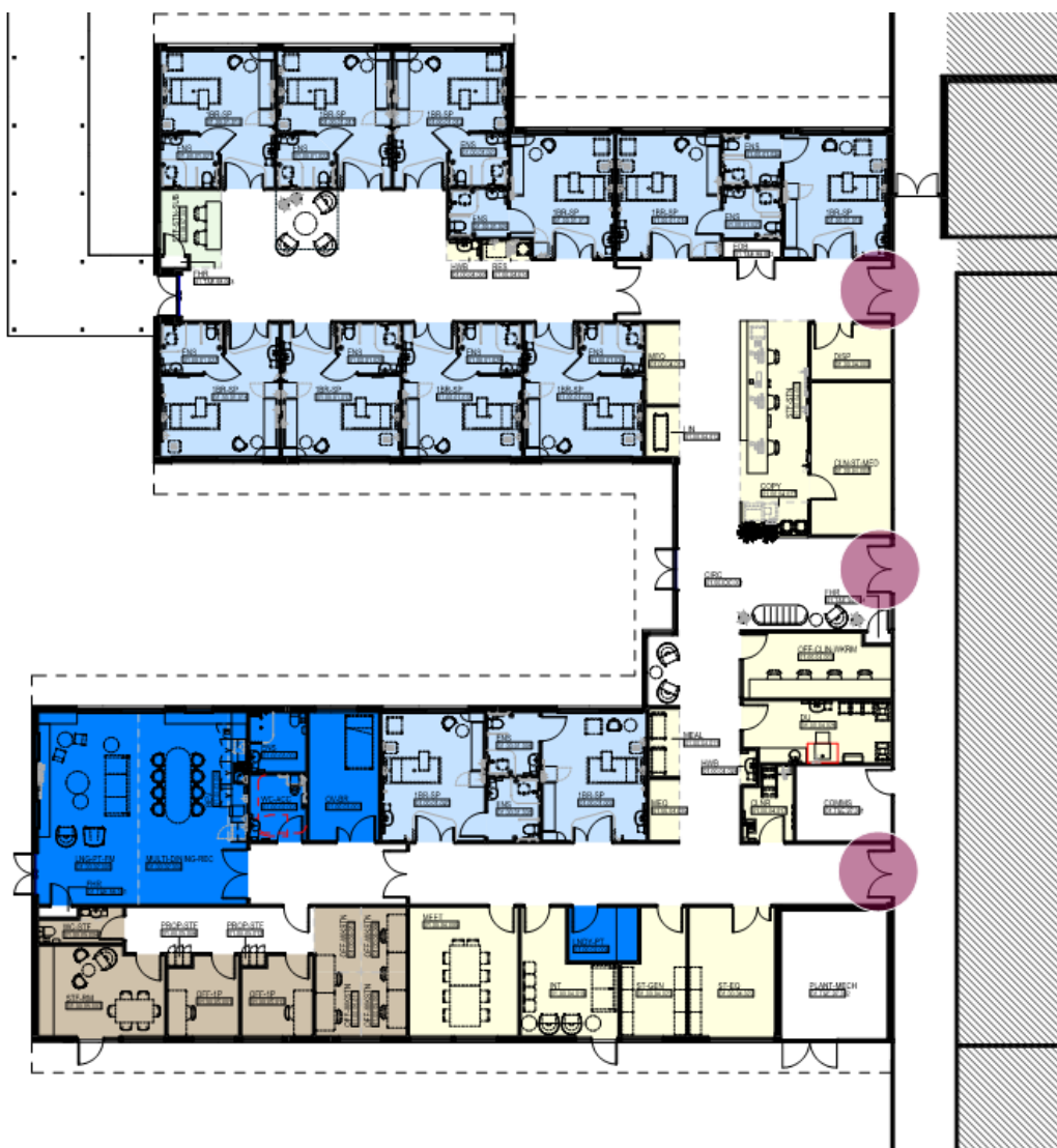
Figure No. 9: Swing of horizontal exit doors against the direction of egress
